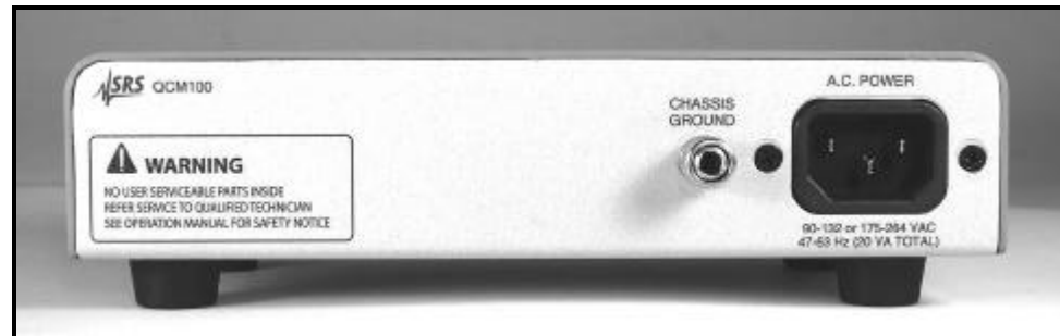
Figure 2. Back Panel of QCM100 Analog Controller.
